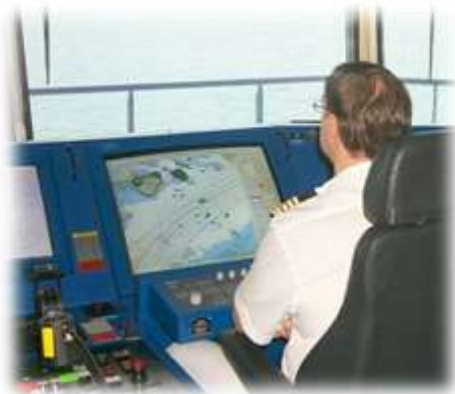
ECDIS and up-to-date ENC's in use at sea
