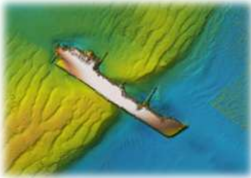
A wreck detected by side scan sonar
